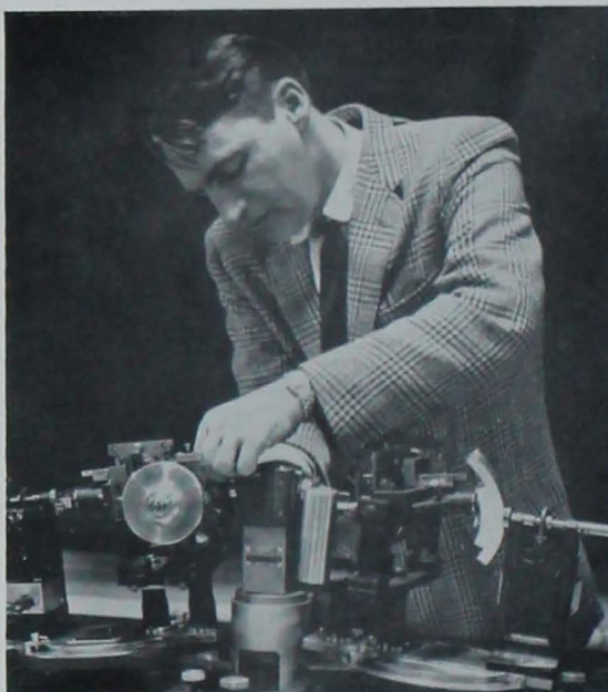
CHEMISTRY PROFESSOR Robert Rundle adjusts an x-ray camera before photographing a crystal.
