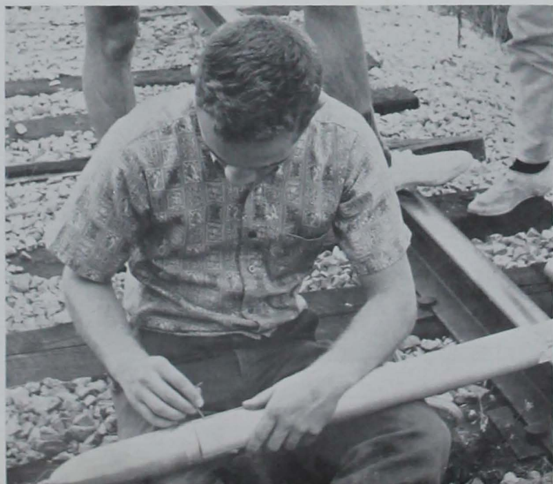
AERO E SENIOR Larry White resets the timing mechanism on an Aero E lab rocket at last summer's rocket shoot.
