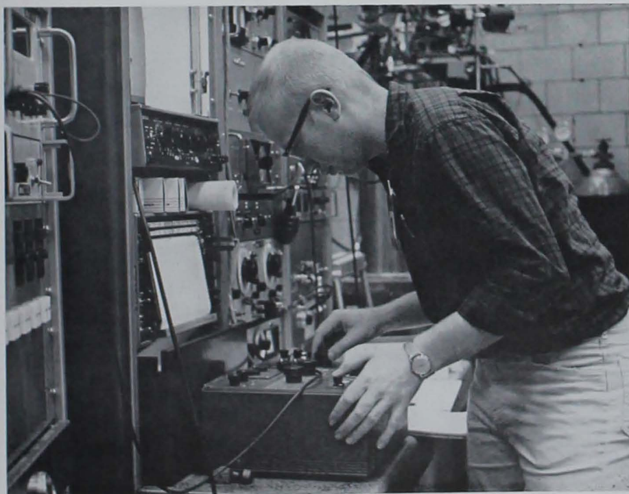
Dave Boyle, Physics graduate, sets the value on a "black box" which controls the strength of a magnetic field set up by superconducting magnet.
