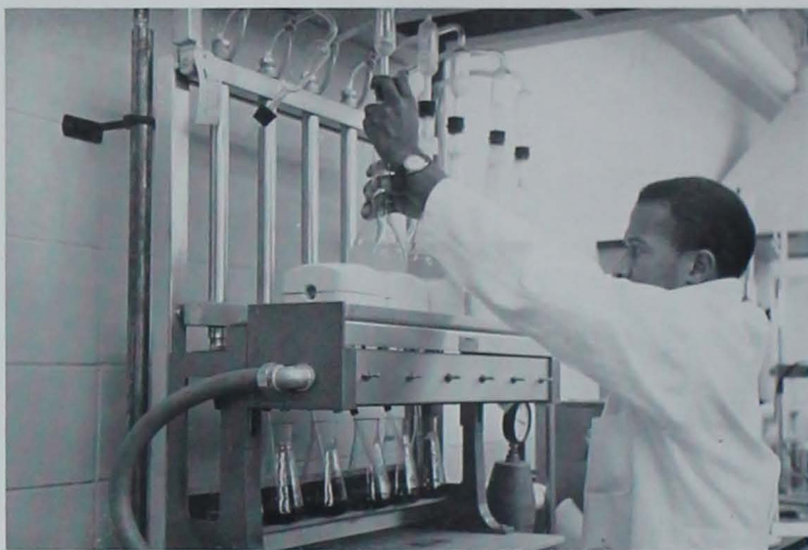
A poultry science grad student works on a Macro-Kjeldahl (protein) analysis as part of research for his thesis.
