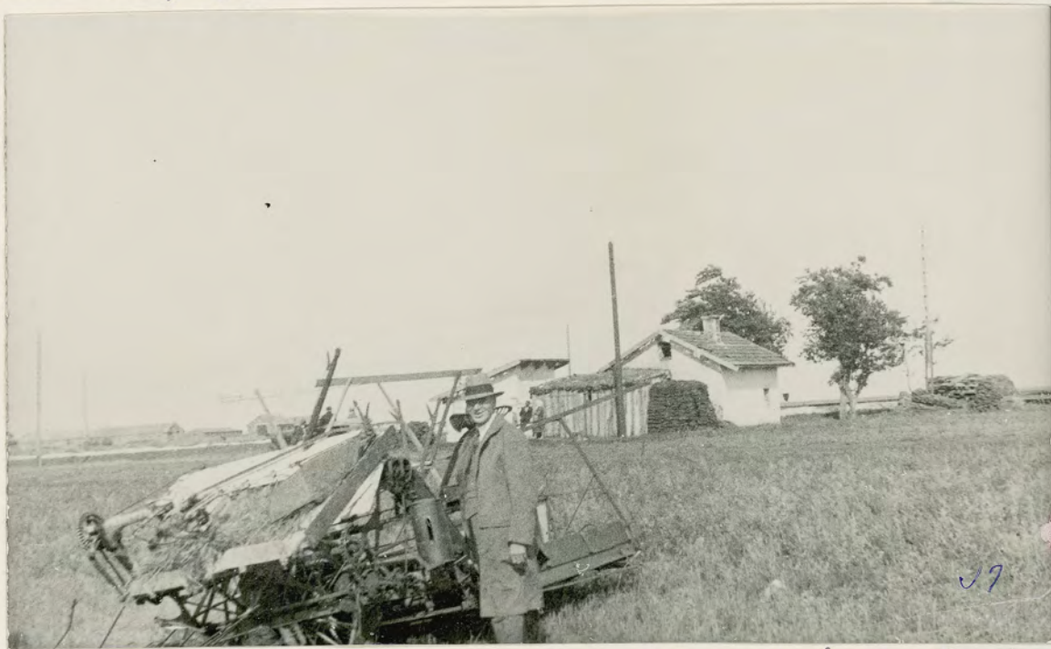
A Russian binder almost an exact duplicate of the McCormick. - On the road from Simferopol
