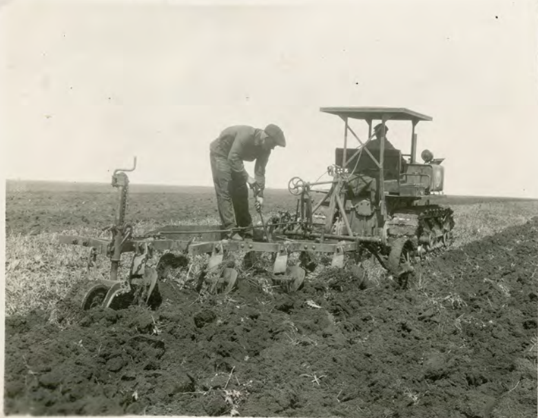
Reg. # 0068799 Cletrac 40 pulling 4 bottom shuttle flow for fallow on Sovhoz No. 2. North Caucasus near Kirov. Soil is heavy, plowed not sown. Man on top of plow uses a spade with which he does maintenance June 29 1929
