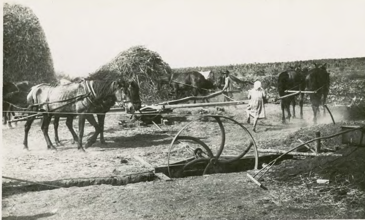
HORSE POWER FOR DRIVING THE THRESHER SHOWN BELOW
