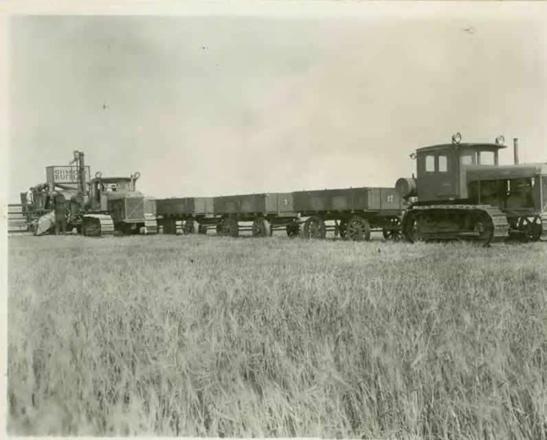
Dumping from combine tanks into a wagon train
