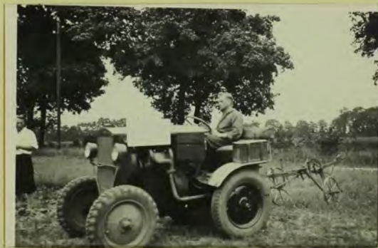
SMALL TRACTOR. DR DENCKER idea of a tractor for Germany, 6-8 HP
