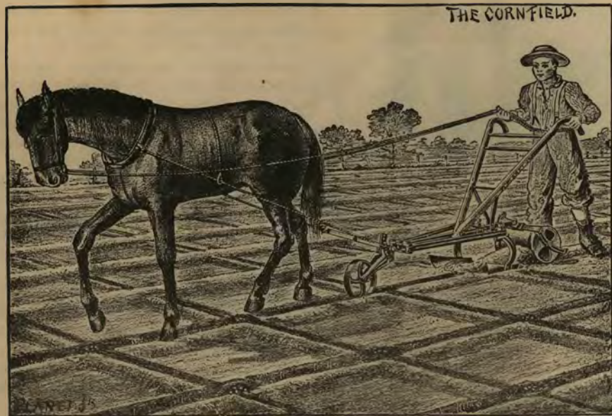
Fig. 36.—The "Planet Jr." Horse Hoe with Covering Attachment.
