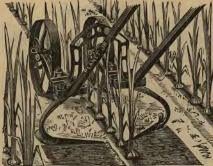
Fig. 11.—Hoeing both sides at once.
