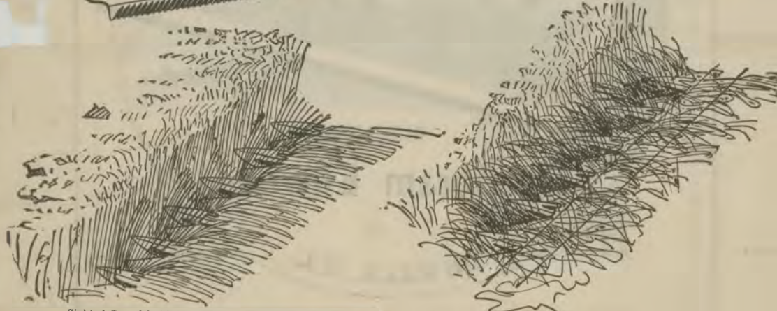
Smooth Guard pushes grass forward, bunching it in being cut, and causes it to fall forward of bar.
