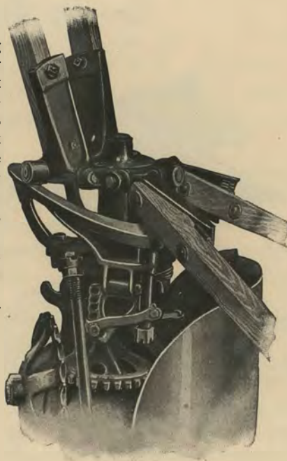
Rake head showing hand latch for controlling the rakes
