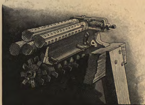
Shredder head and cutter with reversible steel face. Can be reversed quickly and all four edges utilized for cutting
