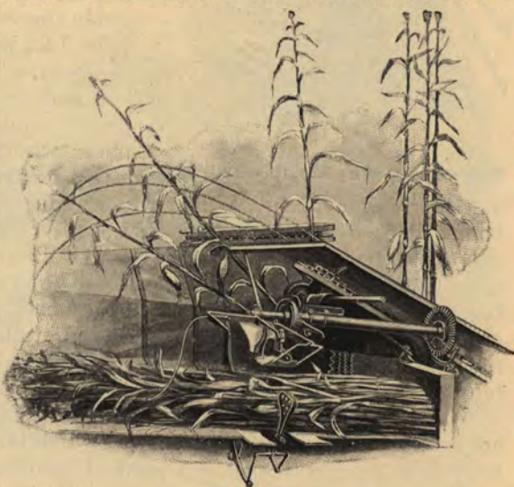
Adjuster set for long corn; band tied far from the butts.
