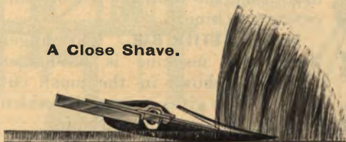
Knife and ledger plate pass each other like blades of shears.
