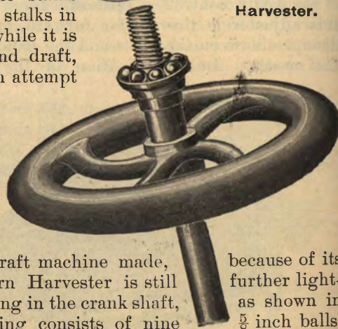
Ball Bearing on Crank Shaft of Deering Corn Harvester.
