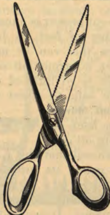
Knife and ledger plate pass each other like blades of shears.
