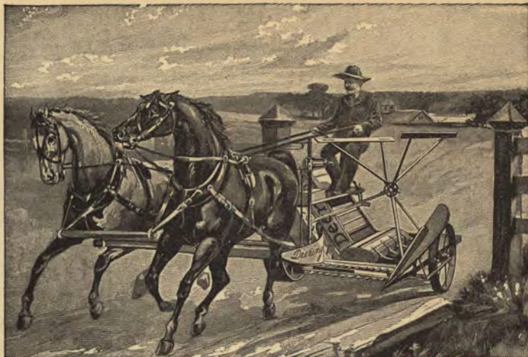
Deering Improved Steel Binder, with Jointed Platform Folded.
