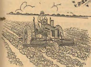
Right: John Deere Two-Row Cultivators for listed crops. Hydraulic power lift.
