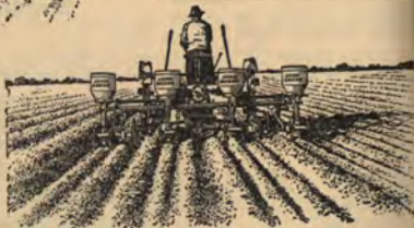
Left: John Deere Cotton and Corn Planter and Equipment. Handles many crops. Fits Models "A", "B", "G" and "H" Tractors. Can be used alone or in combination with cultivator to bed, sweep, or furrow at the same time it plants and fertilizes. For cultivating, substitute shovels. Variety of planting equipment available.
