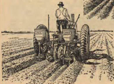
Right: Four-row planting attachment for John Deere Bedder. Also used as two-row,
