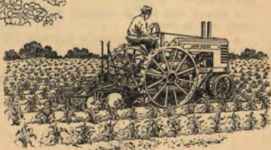
Right: John Deere Two-Row Cultivators for listed crops. Hydraulic power lift.
