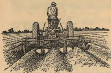
Right: John Deere Two-Row Middlebreaker for listing, relisting, bedding, middlebreaking, sweeping beds, and reworking middles.
