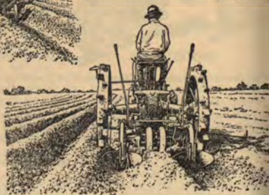
Left: John Deere Cotton and Corn Planter and Equipment. Handles many crops. Fits Models "A", "B", "G" and "H" Tractors. Can be used alone or in combination with cultivator to bed, sweep, or furrow at the same time it plants and fertilizes. For cultivating, substitute shovels. Variety of planting equipment available.
