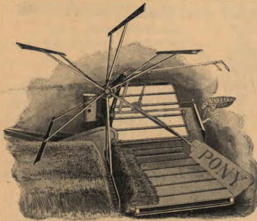
Pony Reel, back and down for short grain.
