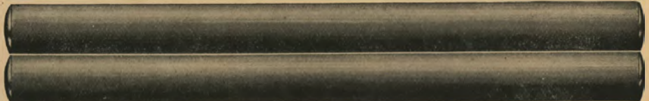
Exact size of rollers in bearings of main wheel of Deering Pony Binder.
