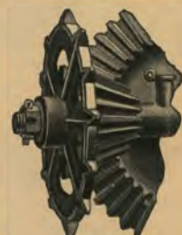
Threaded Nut for keeping Crank Shaft Sprocket in perfect mesh.
