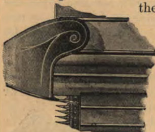
Elevators extend seven inches in front of the knife.
