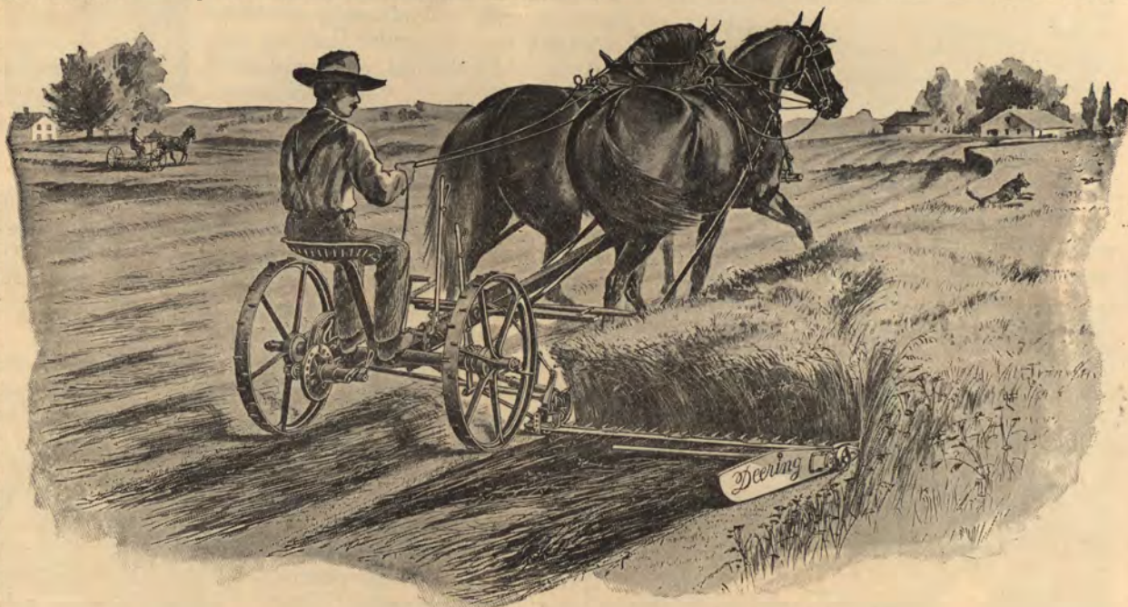
THE DEERING IDEAL MOWER, 4½ and 5 ft. cut, with Roller and Ball Bearings throughout.
