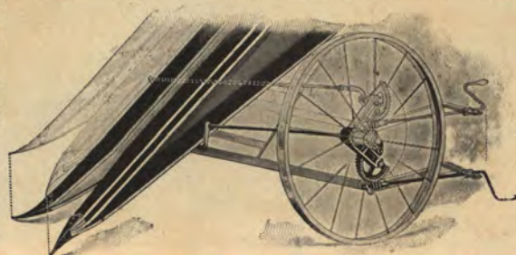
Raise and Lower Device—Points always level.
