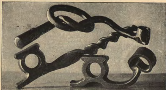
Ideal Steel Pitman and Knife-Heads Tied in a Knot and Twisted Cold.
