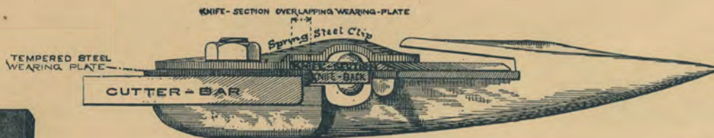
The Perfect Cutting Apparatus of the Deering Mowers. Steel Against Steel Everywhere.
