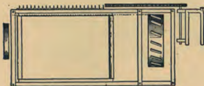
PLAN OF FRONT GEARED BINDER.
