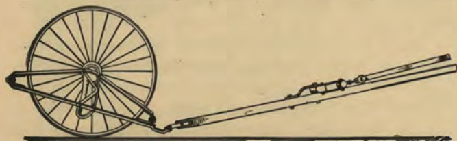
The Line of Draft of the Deering Harvester is Near the Ground.
