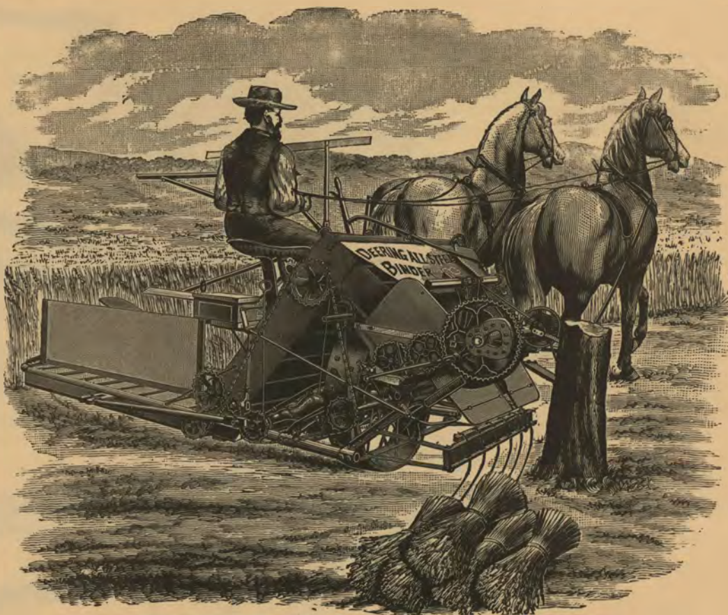
THE DEERING STEEL BUNDLE-CARRIER FOLDED FOR PASSING AN OBSTRUCTION
