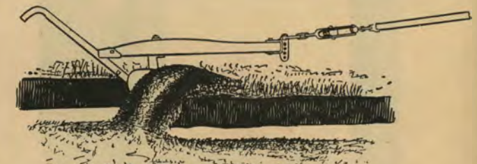
The high point of draft throws the plow deep into the ground. The same principle applies to the Harvester.
