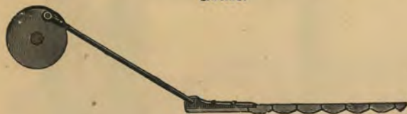
Here half the power exerted tends to pull the sickle upward out of the guards. Wears the sickle out in a short time and causes a noisy, jerking motion annoying to the driver, fatal to the machine, and severe on the horses.
