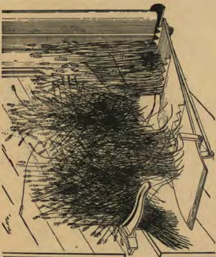
The Vibrating Butt Board as a threshing machine.
