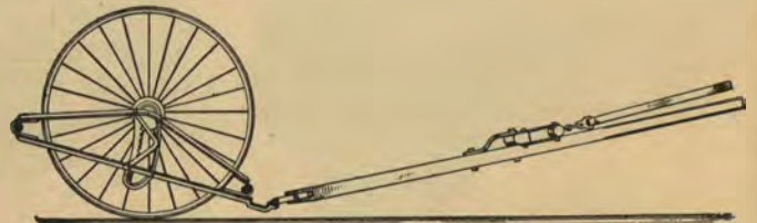
The point of draft for the Deering Harvester is near the ground. This makes light draft and destroys neck weight.
