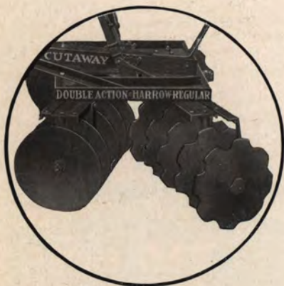
Double Action Harrow equipped with solid disks front and cutout disks rear
