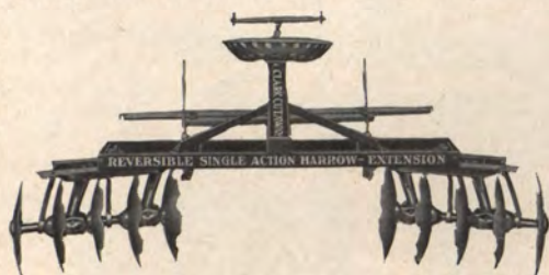
Reversible Single Action Harrow—Extension with Gangs Reversed
