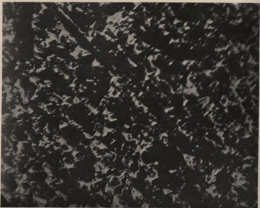
This photomicrograph shows the internal structure of a CUTAWAY forged-edged disk, illustrating what our forging process does to the steel. Note the contrast between this and the upper photomicrograph. Read Prof. Upton's article.
