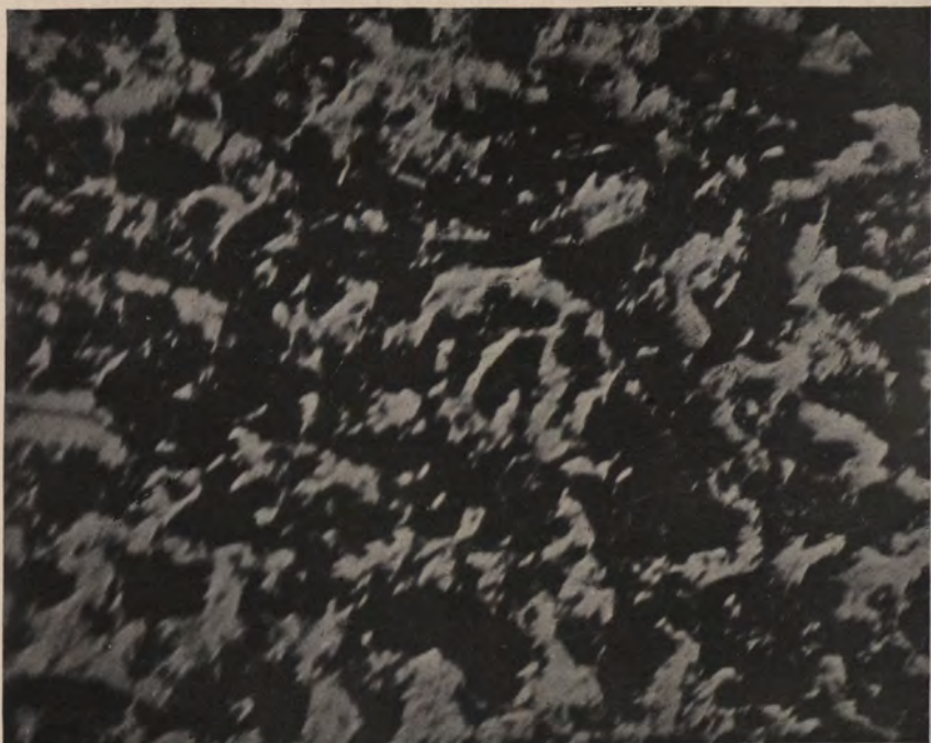
The above photomicrograph shows the internal structure of disk steel not forged. See article on page 9.
