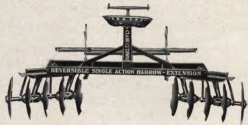
Reversible Single Action Harrow — Extension with Gangs Reversed. To reverse, it is only necessary to drop the lever links, swing the gangs around on the king bolts and reattach the links.
