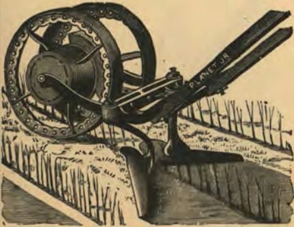
Fig. 5—The "Planet Jr." Combined Drill and Wheel Hoe, hoeing both sides of the row.
