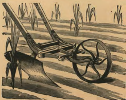
Fig. 21—The "Planet Jr." Single-Wheel Hoe as a Plow.
