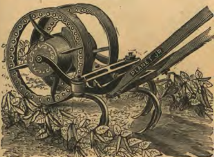
Fig. 7—The "Planet Jr." Combined Drill and Wheel Hoe, as a Cultivator.
