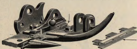
Adjustable Hard Steel Bearings for the Scythe Head
