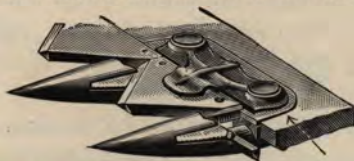
Steel Adjustable Wearing Plates
