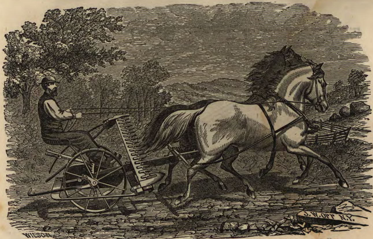
The Cutter Bar folds over the Tongue, making the Climax as Portable as a Sulky.
