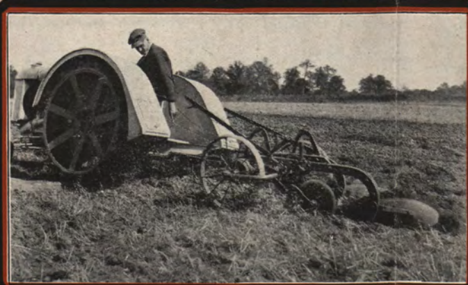
Tractor wheel going over obstruction does not affect the even depth of the plow.
