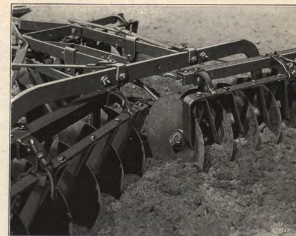
Offset Construction of Rear Gangs Leaves No Ridge
