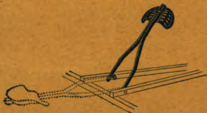
SHOWING METHOD OF ADJUSTING SEAT. Seat in Natural Position and Thrown Forward Out of the Way.
