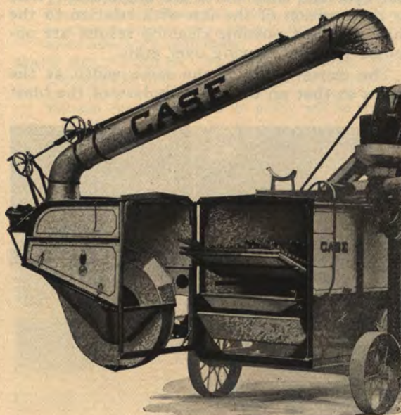
Hinged Windstacker on 22x36 and 28x46 Facilitate Working Inside the Machine
