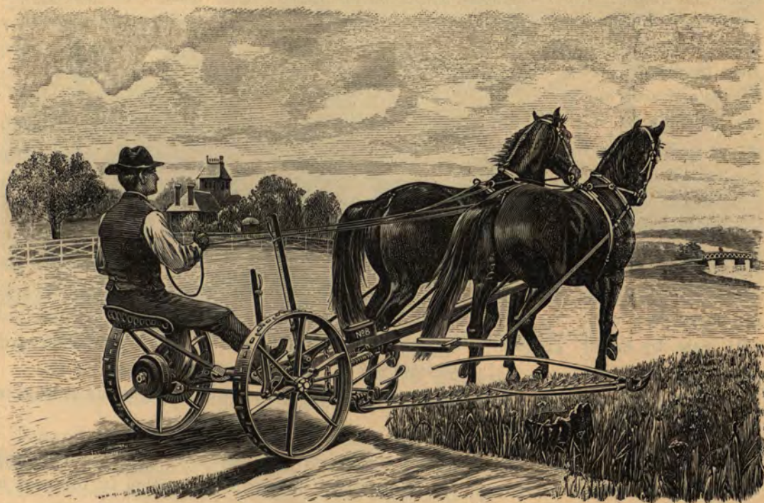
ON THE ADRIANCE MOWER THE BAR IS EASILY OPERATED BY DRIVER'S FOOT.
