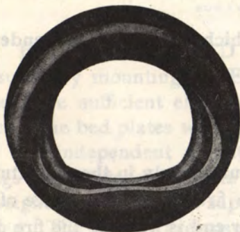
Compressed section of Tube showing ductility.
