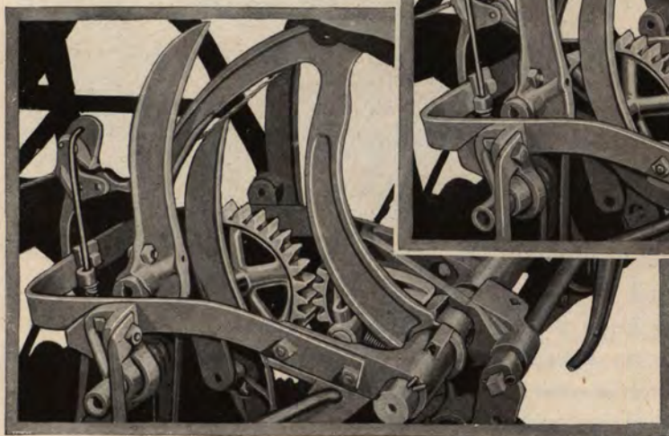
Packers "out of gear" as needle enters breast plate. Note as needle carries twine upward, the tension is applied automatically.
