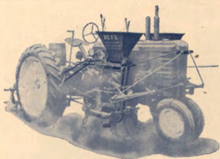
McCormick-Deering Model "H" Tractor with 2-Row Planting and Cultivating Rigs and BLUE DISTRIBUTOR.
