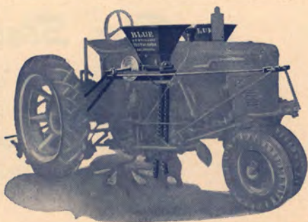
John Deere Model "B" Tractor with 2-Row Planting and Cultivating Rig and BLUE TRACTOR DISTRIBUTOR.
