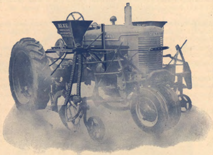
McCormick-Deering Model "M" Tractor with 3-Row Middle Breaker and BLUE DISTRIBUTOR.
