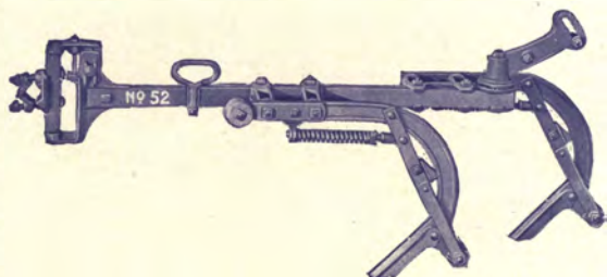
No. 52. This style of Gang is built for Walker Cultivator only, has curved shank new style Spring Trip, Four Shovels. Cut shows slotted boot, but is made either with round or slotted boot. Weight 131 pounds per pair.
