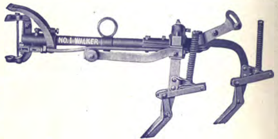
No. 1. This is the same as the No. 1-B gang, except it is made for walking cultivator frame only, the pipe beam of the No. 1 being a few inches shorter than on the No. 1-B. Weight with shovels 160 pounds per pair.
