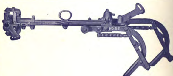
No. 55. Four Shovel, Spring Trip, Curved Shank, Pipe Beam, parallel, can be furnished in round or slotted boot, made for Walking Cultivators only. Weight with shovels complete 134 pounds per pair.
