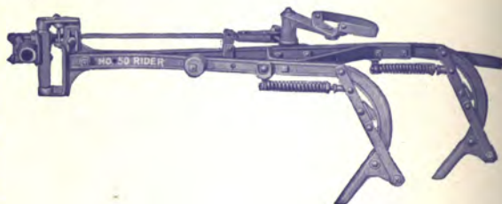
No. 50. For Rider. Made like Walker Gang with the addition of Lateral Guide. Furnished with either Round or Slotted Foot. Weight 130 lbs.
