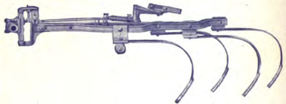
No. 10. With Lateral Guide. Eight Shovel, Spring Tooth, made in either round or flat boot, can be used on Pilot, Rider or Walker frames. Weight complete with shovels 97 pounds per pair.
