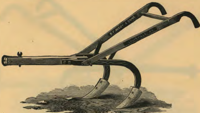
WOOD BEAM, IRON STANDARDS.
