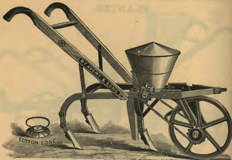
No. 1. SHOWING COTTON CONE AND REGULAR BLADE COVERERS.
