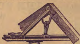
Showing End Brace used with Solid Steel Track when Hay is taken in at end of barn.
