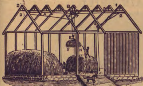
The Adjustable and Reversible Porter Carrier put up to carry hay on either side.
