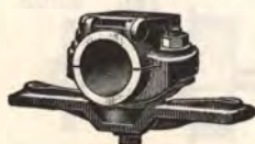
PIVOTED BOX NEXT TO PULLEY.
