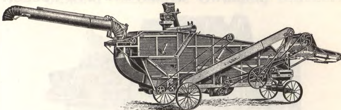
The Columbia with Parsons' Self-Feeder and Wind Stacker.
