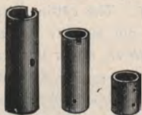
BRASS BUSHINGS ON THE BUCKEYE.
