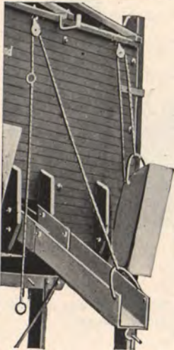
25-TON PORTABLE BIN WITH FOUR-SECTION REVOLVING SCREEN Lowered on Wagon for Moving
