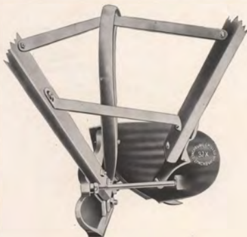
Rear View of Lynchburg Chilled Plows Showing the "Lynchburg" Special Bracing
