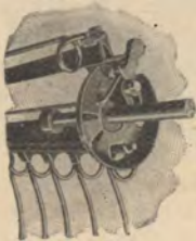
End of Rake Head showing operation of ratchet.
