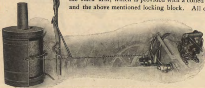
Twine from Twine Can to Knotter.
