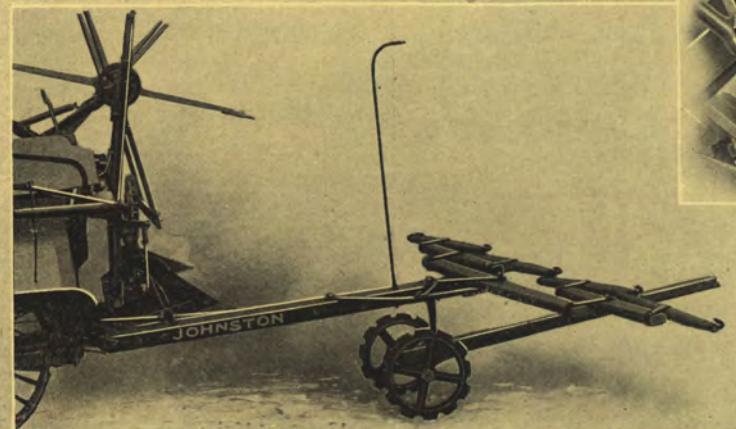
Bundle Carrier, folded and extended. Binder on Truck. Truck Axle Fastenings, inside and out. Steel three-horse Equalizer. Tongue Truck for 7 foot and 8 foot machines.
