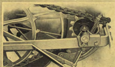
Main Frame in one piece. Elevator Frames. Main Wheel. Roller Bearings. Gearing and Brass Bush. Chain and Tightener. Raising Apparatus.
