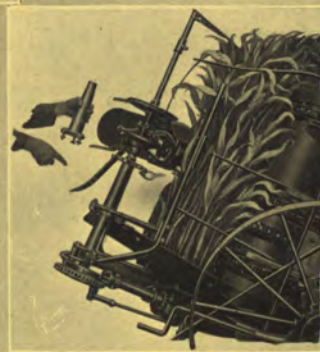
Showing Frame, Wheels and location of Pole and Seat. . . Forty inch Wheel, Roller and Brass Bush Bearings. Main Drive Gears. Cutting Apparatus. Conveyor Fingers. Adjustable Chain Tighteners. Separate Idler Sprocket Box. Binder Attachment. Automatic Gates. Set for Short Corn.
