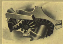
Elevators. Separate Roller Box. Canvas Tightener Levers for Elevators and Platform Binder Attachment and Gearing. Seventh Roller. Tier Frame Support.
