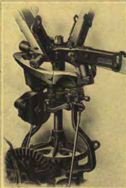
Reaper Gearing, Roller Bearings, Grain Wheel and Outer Divider. Raising Lever and Suspending Bar. Rake parallel with Bar. Automatic Trip. Rake Standard. Platform Support and Braces. Reaper Folded.
