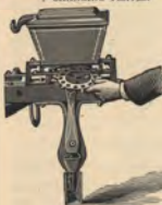
OPEN SEED VALVE—CORN SEEN IN ADVANCE OF THE HILL.
