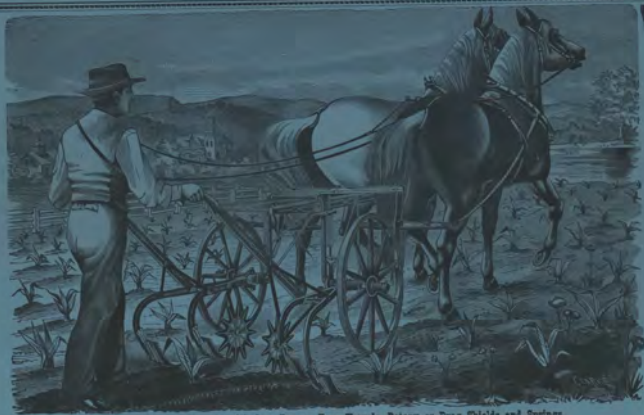
No. 1.—Walking Cultivator with Iron Beams, Four Shovels, Rotary or Drag Shields and Springs.
