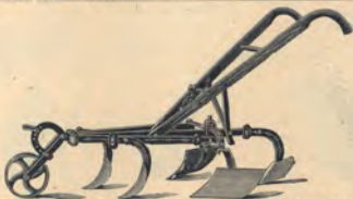
BUCKEYE ONE-HORSE FIVE-SHOVEL CULTIVATOR WITH ATTACHMENTS ON.
