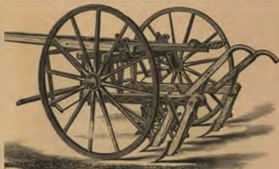
No. 6—New Junior for 1883 with Wood Beams, 4 Shovels, Rotary Shields and Treadles.
