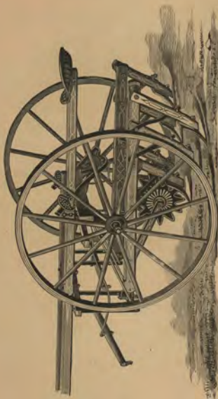
New Buckeye Senior Cultivator with Rotary Shields and Treadles.
