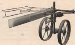
Illustration—showing pole set straight for two or four horses. For three horses, loosen set screw and slide shaft as indicated by dotted lines, then secure with set screw
