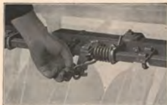
The scraper spring tension can be changed without using any tools
