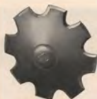
View of the cutaway disk—can be had on any harrow (see pages 8 and 11).
