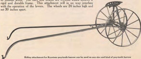
Riding attachment for Keystone peg-tooth harrow can be used on any size and kind of peg-tooth harrow
