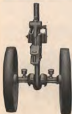
Front view of the forecarriage arranged for use without a pole. This view shows very clearly how the wheels are swiveled to follow the unevenness of the ground
