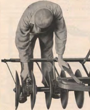
It is easy to grease from the rear of the harrow
