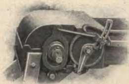
Detail illustration showing improved feed mechanism and method of changing length of cut.
