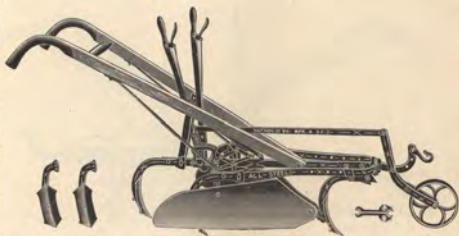
IMPROVED NO. 31 DOUBLE LEVER CULTIVATOR WITH LONG HILLERS.
