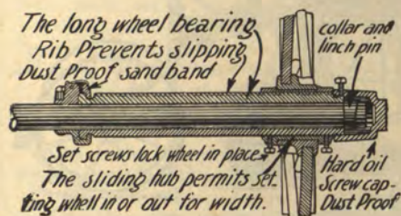
The Adjustable Wheel Box used on our Sulky Listers
