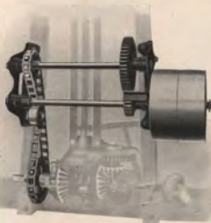
No. 442 Engine Driving Jack Attached to Wagon Dump
