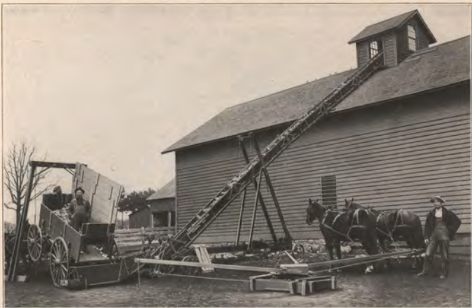
A 48-Foot Elevator Outfit (with Swivel Hopper), Delivering into Cupola
