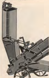
Tilting Hopper Swung Upright to Permit Wagon to Pass to Position for Unloading
