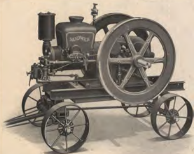
Sandwich Four-Horse Power Hand Portable Kerosene Engine
