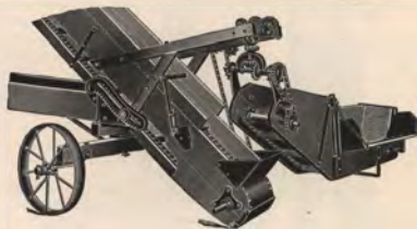
Swivel Hopper Swung at Right Angle and Out of Way of Wagon
