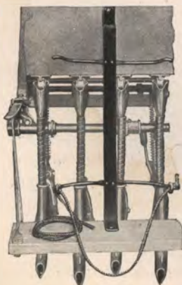
Sack-rack attached to foot-board and grain-box
