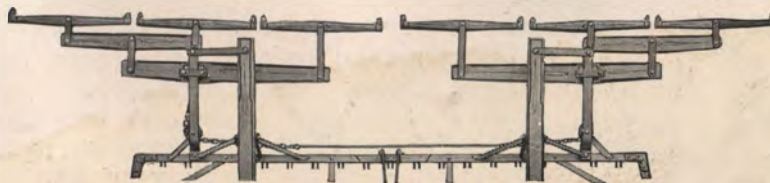
Six-horse chain equalizer hitch, two poles
